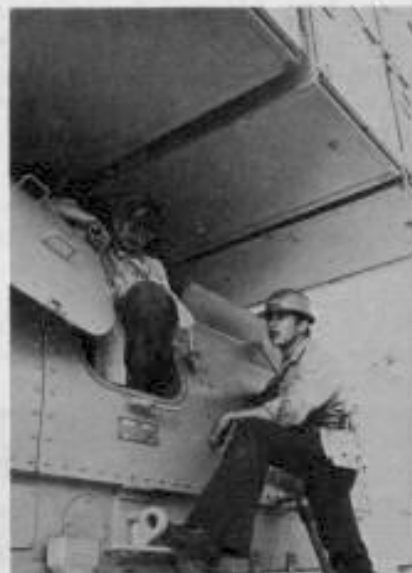
Gunner's Mate (Torpedoes) Second Class Jim Plansky and Gunner's Mate (Torpedoes) Seaman Apprentice Breck Crandell climb out of the Anti-Submarine Rocket (ASROC) launcher carriage, which houses the launcher's rotation and elevation power unit. ASROC, located on the forward main deck between the superstructure and the Terrier missile launcher, uses missile-launched torpedoes to seek out and destroy underwater targets.
