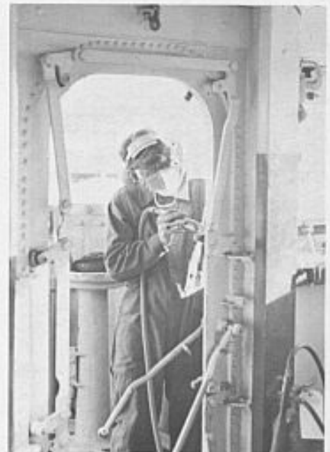
Dressed in protective clothing, Quartermaster Seaman Walker Smith chips paint from a water-tight door on the port (left) side of the bridge.
