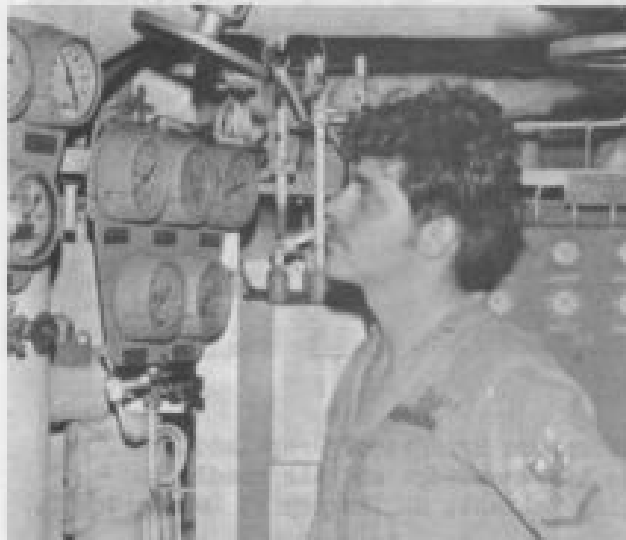
FN Reynolds of East Orange, N.J. here checks feed pump pressures in the fire room to ensure that everything is running normally.
